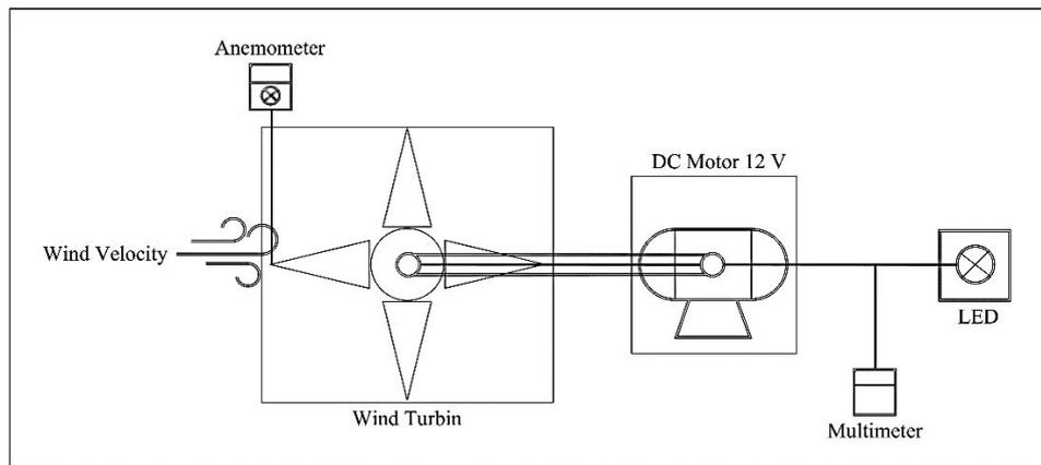
**Figure 2. PLTB prototype system testing configuration**
