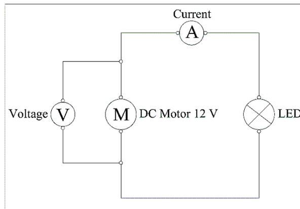
**Figure 3. The Circuit of Current and Voltage Measurement**
